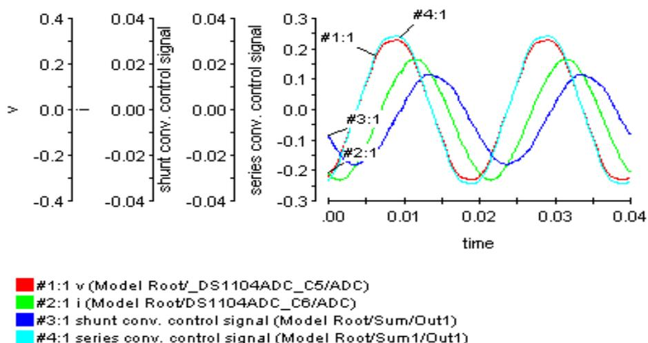
Fig.6. control series and shunt converter control waveforms for case (1), input current (i), input voltage (v).
