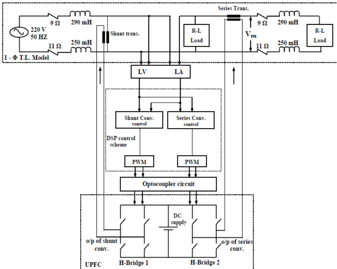
Fig.4. Configuration of Single phase UPFC system
