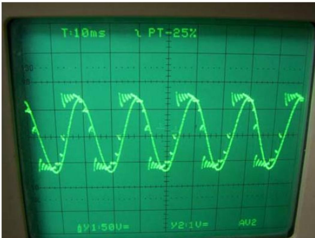
Fig.11. Case (2) series converter Output voltage and measured input current waveforms
