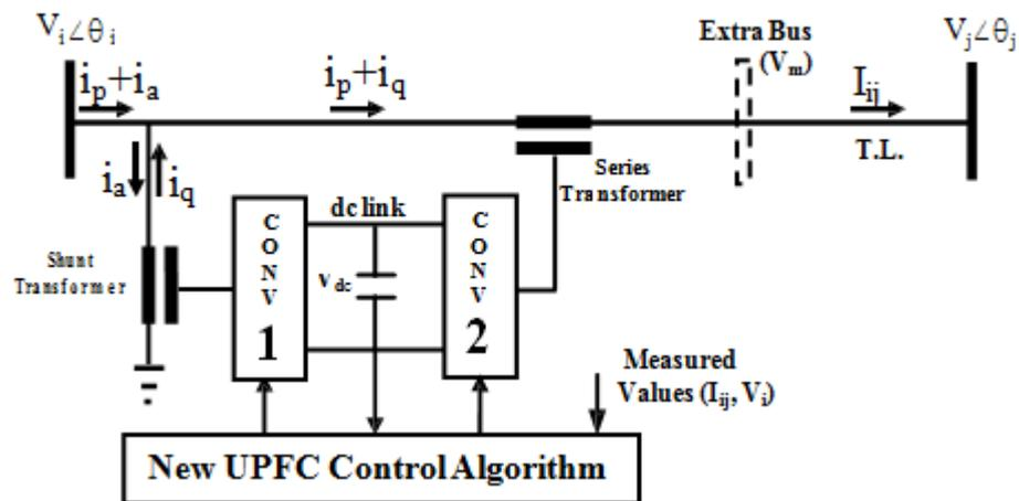
Fig.1. New UPFC Control Algorithm
