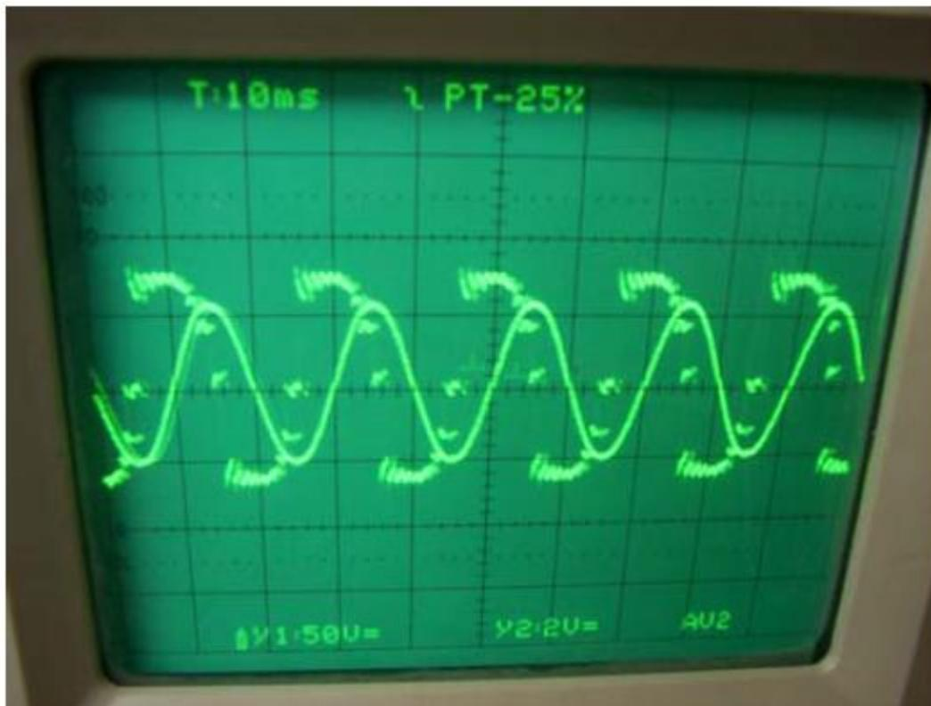
Fig.10. Case (2) shunt converter Output voltage and measured input voltage waveforms
