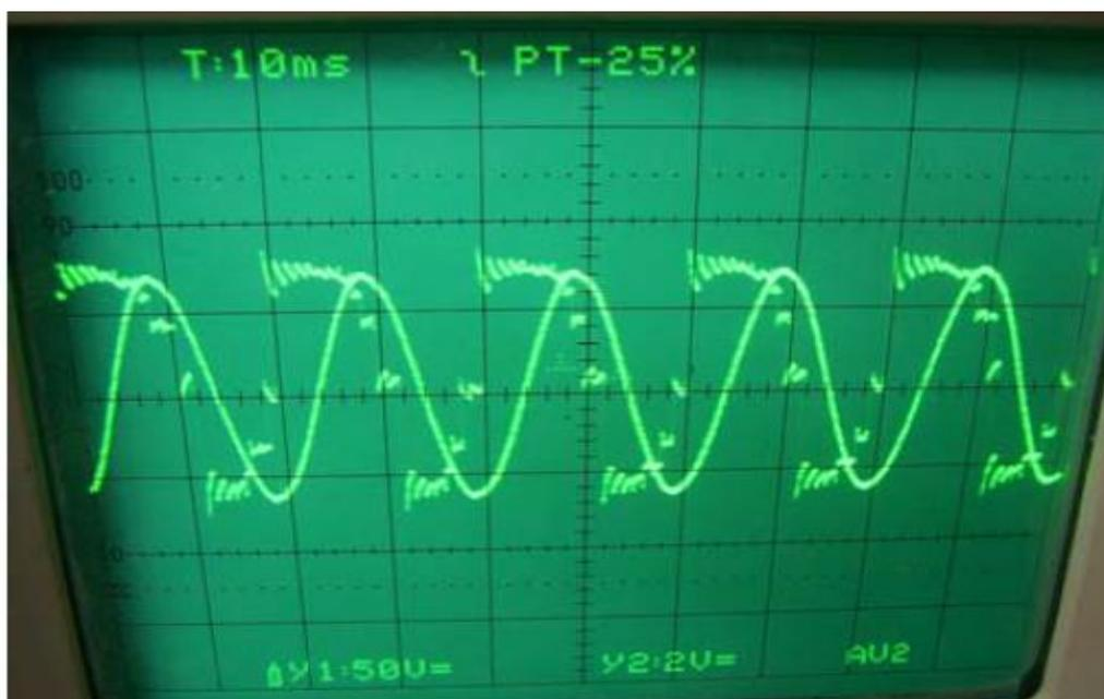
Fig.8. Case (1) shunt converter Output voltage and measured input voltage waveforms
