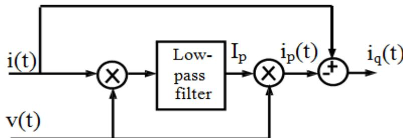
Fig.2. calculating the UPFC shunt injected current by using Open-loop system.
