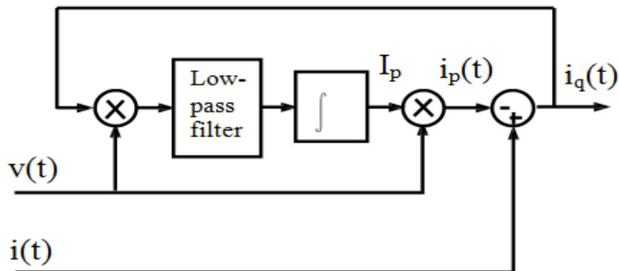
Fig. 3. UPFC shunt injected current Closed-loop system
