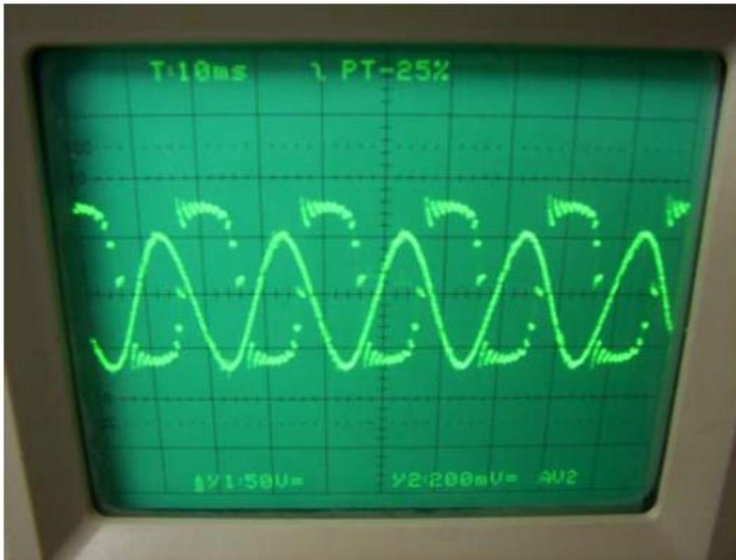
Fig. 9. case (1) series converter Output voltage and measured input current waveforms
