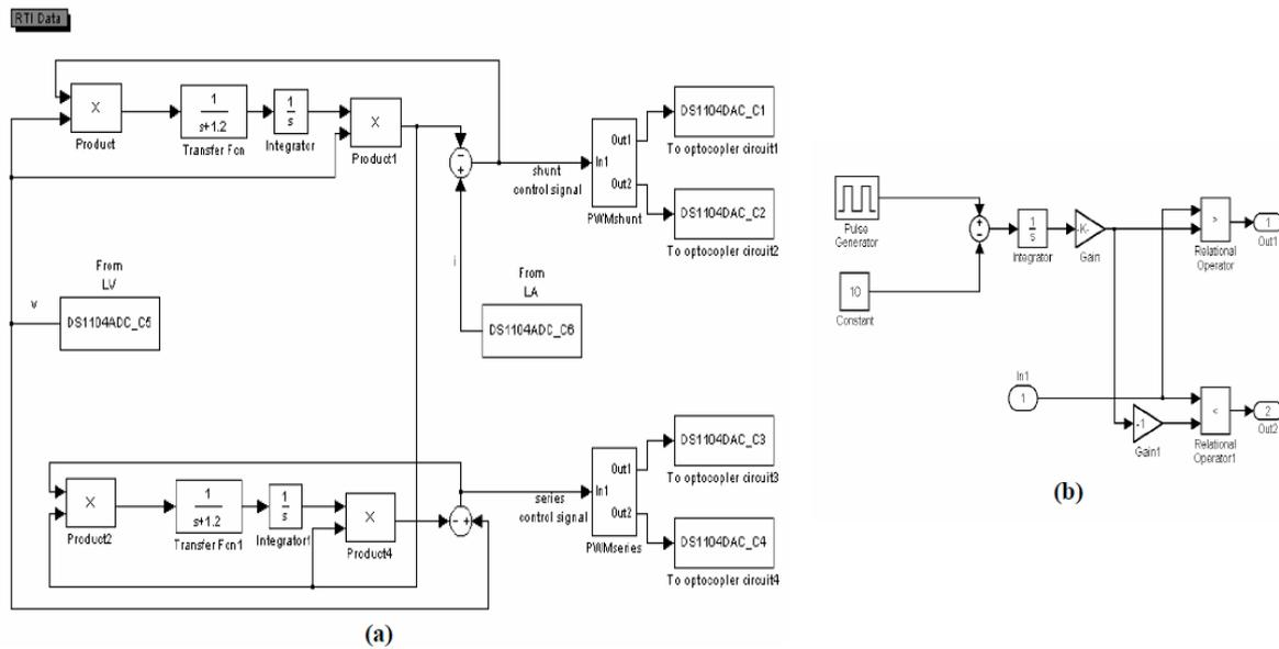
Fig.5. (a) Single phase UPFC Control algorithm
